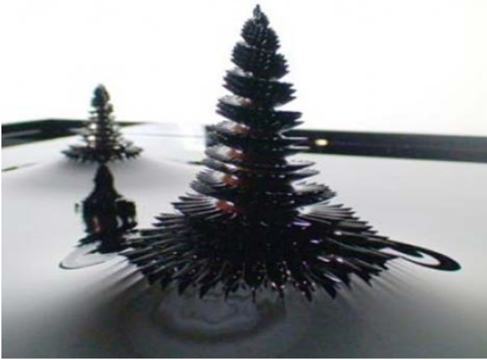
Ferrofluid on glass, with a magnet underneath.
