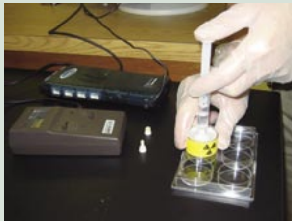
FIGURE 2 Student eluting Ba-137m isotope into a well plate from an isogenerator capsule with dilute salt solution.
